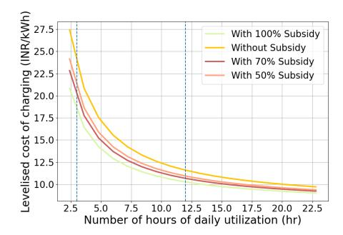
Figure 17: The effect of subsidies on the LCOC at the model EVCS (cost of grid electricity = INR 5/kWh for all cases)
