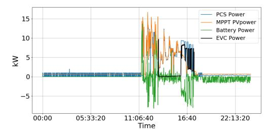
Figure 10: Energy and charging profiles logged in the PCS during its operation on 1 September 2020
