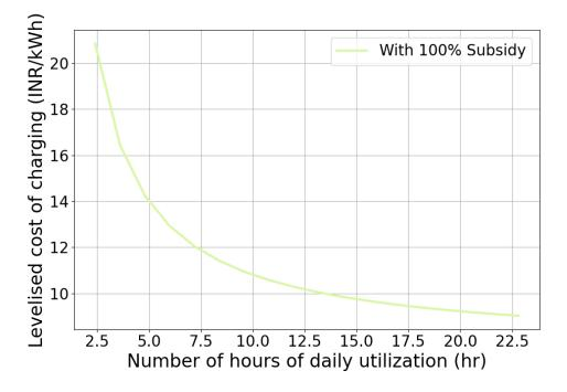
Figure 16: LCOC for the model EVCS as a function of daily utilisation of chargers. The x-axis denotes the number of hours of operation per day for each charger in the EVCS. It corresponds to 100% subsidy on the capex of EV chargers and for the grid electricity cost of INR 5/kWh (as in Karnataka).
