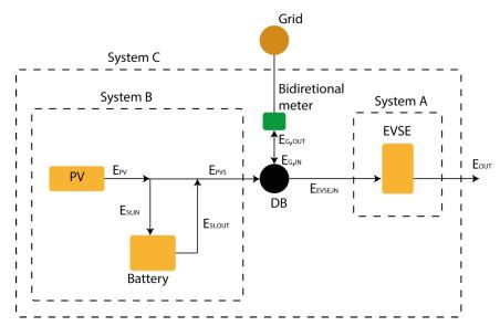
Figure 15: Block diagram used for the techno-economic modelling of solar- plus energy storagebased EV charging. DB represents the distribution box.
