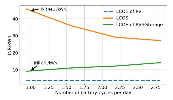
Figure 20: Levelised cost of solar PV plus storage plant along with the same for subcomponents (PV only and storage only) as a function of battery utilisation. The PV plant and storage sizes are maintained constant throughout the calculations. The values highlighted with arrows are used in the analysis in the subsequent sections.
