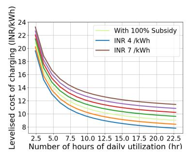
Figure 19: The effect of different electricity tariffs on LCOC (with 100% subsidy on EVSE). The bottom-most and the top-most figures correspond to INR 4 and 7/kWh, respectively. The intermediate curves represent increments by INR 0.5/kWh from the bottom to the top.
