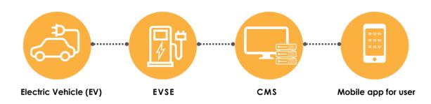
Figure 1: These are the main components of a public EV charging station. EVSE stands for "electric vehicle supply equipment", and CMS stands for "central monitoring system". Main entities in the infrastructure:
