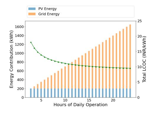
Figure 22: The variation of the levelised cost of charging (LCOC) of EVCS connected to an RTPV system without energy storage (line plot). The bar graphs represent the mix of solar and grid energies.
