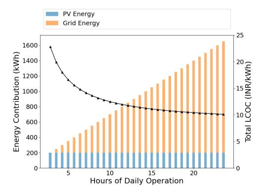
Figure 21: The variation of the total levelised cost of charging (LCOC) of the model EVCS connected to a solar plus storage system (line plot). The bar graphs represent the mix of solar and grid energies.
