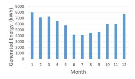
Figure 3: Monthly PV energy generation data from simulation for the 40 kWp RTPV system (for the year 2020)
