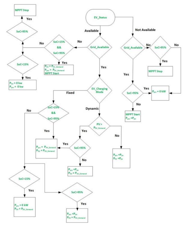
Figure 8: Source prioritisation algorithm for RTPV- and battery-coupled EV charger. Parameters' meaning – SoC: state of charge, P<sub>EV</sub>: power demand from the EV, P<sub>PCS</sub>: power delivered by the PCS, P<sub>PV</sub>: power delivered/generated by the solar panels
