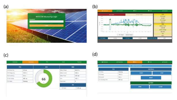
Figure 9: Snapshots of the user interface to the PCS for remote monitoring: (a) the user login page; (b) the dashboard showing the energy profiles related to PV generation, battery energy, and the total PCS energy as a function of time of day; (c) the display of certain parameters related to the PCS power and battery SoC; and (d) certain system-level controls in the same interface
