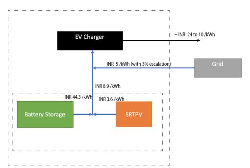
Figure 24: Schematic showing the costs associated with different subcomponents of the gridconnected RTPV-based EVCS
