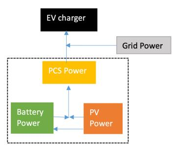
Figure 13: The schematic of the energy/power flow from various components to the EV charger
