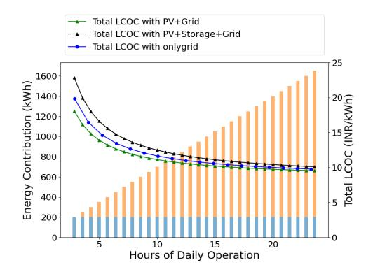
Figure 23: The comparison of the levelised cost of charging (LCOC) from the model EVCS for the three cases: with RTPV only, with RTPV and energy storage, and just the EVCS alone. All the calculations involve replacements of components (chargers and inverters) over a time of 25 years (= RTPV life). The bar graphs show energy contributions from the grid (orange) and the RTPV system (blue).
